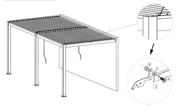
Mark holes for expansion bolt  $0 \times 4$  on each post.
