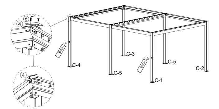
Attach all eight gutters B-1X4,B-2X2,B-3X2 by hooking inside the A-1,A-2,A-3 beams.
