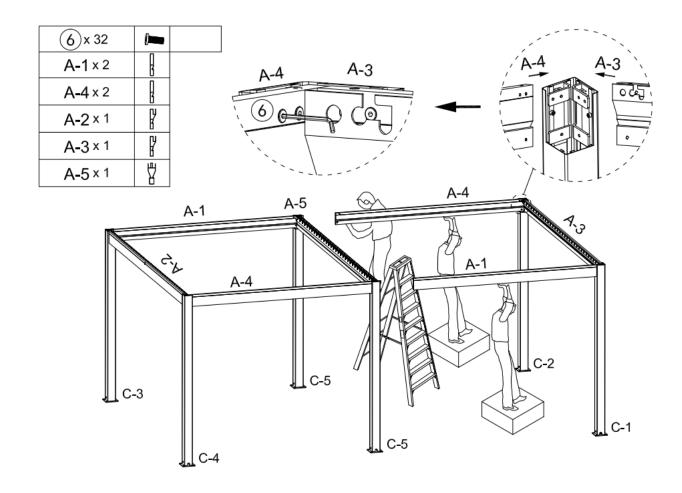
Use bolts 6x4 to fasten beam 1 & beam 4.
