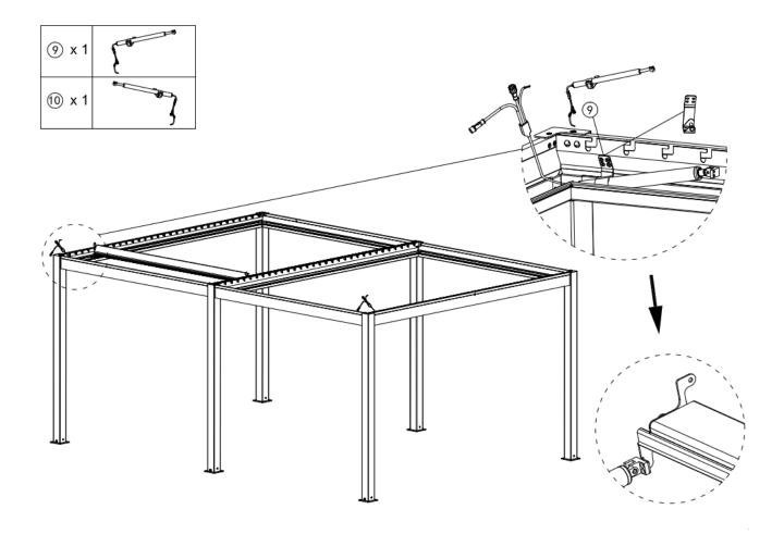
Fasten (12)x4 gutter connector and (13)x2 (50 to 40 connector). Connect the female and male plugs for the LED lighting (DC24V to DC24V) and motor (DC24V to DC24V) and plug the power cable into local socket.
